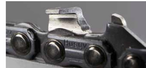
Backward leaning angle. The cutting tooth is filed too high up, making it cut poorly. Use the depth gauge and re-file the cutting teeth according to the recommendation.
