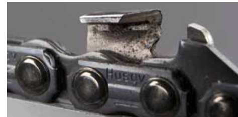
Here you can see how it looks when a cutting tooth is blunt. It is high time to sharpen the cutting teeth. Notice the cutting tooth's "white" edge.
