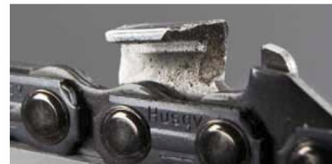
The cutting tooth that has sawn through stone shows an irregular edge where the top layer of the cutting tooth is damaged. It is important that all the damage is filed away to ensure the best possible sharpness.
